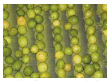
The Brown Oil Extractor (BOE or Brown) process extracts the oil from the fruit first by gently puncturing the flavedo, or peel, of the fruit with thousands of stainless steel needle points.
