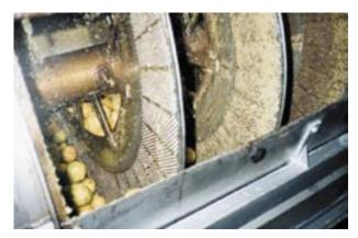
The Pelatrice-style rasper is the third main method of processing, in which the fruit is subjected to rolling disc graters that allow the flavedo to be rasped.
